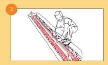
Dig a trench with adapted measures (10cm around the channels). Realise the concrete bedding according to the required depth.
