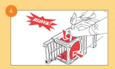
Hammer the desired outlet in and put into position the required outlet/stop end fitting.
